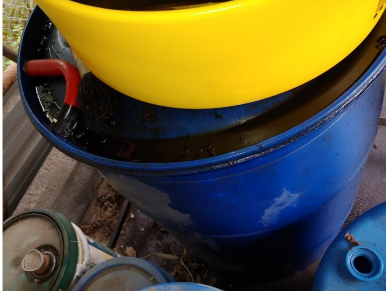
Figure 15-15. Used oil disposal drum with standing oil on the lid at the Freeman Creek Campground maintenance area
