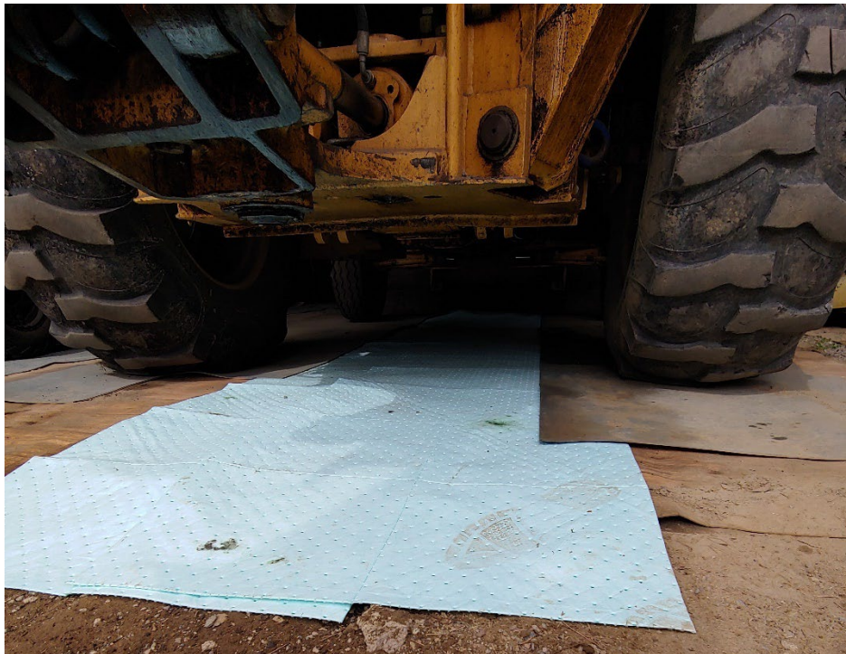
Figure 15-28. Vehicles parked with absorbent pads underneath in the vehicle storage shed at Freeman Creek Campground
