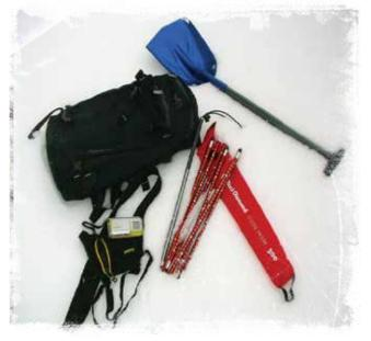
Collapsible probes are also easy to carry along and usually consist of two-foot lengths of tubular steel that join together to make a probe six to twelve feet long. A probe length of less than eight feet is not recommended. Probing is essential to finding a buried victim if there are no visible clues on the surface.
